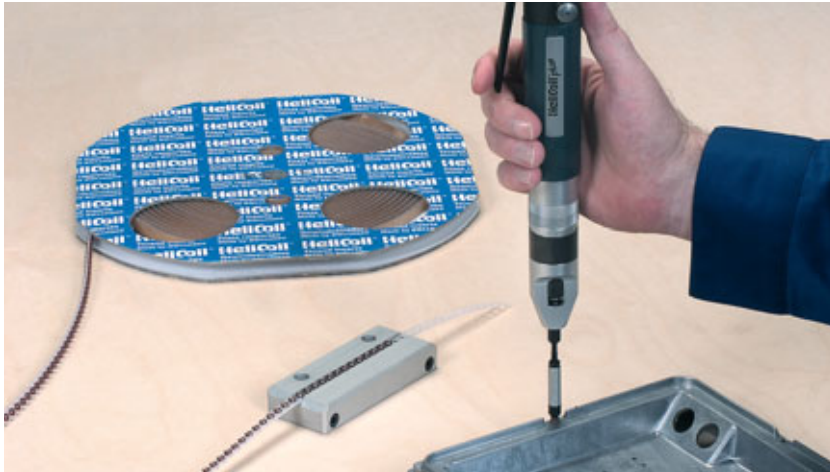
Installation of HELICOIL® Plus
